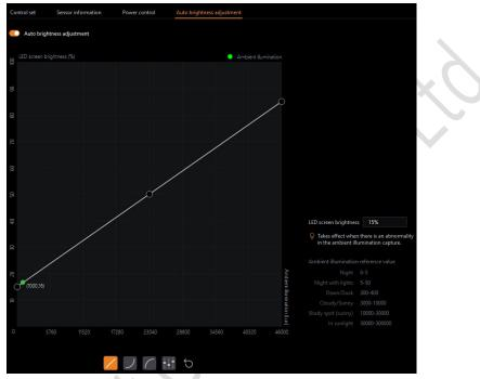
Figure 17.5-1 Auto brightness adjustment interface
