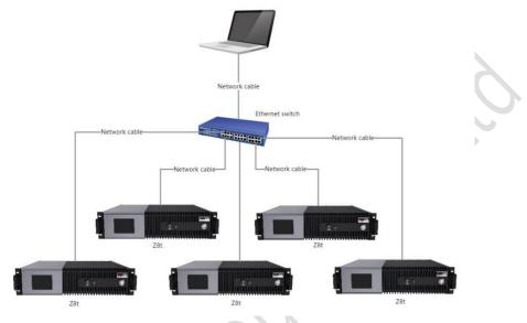
Figure 3.1-1 Multiple processor connection diagram
