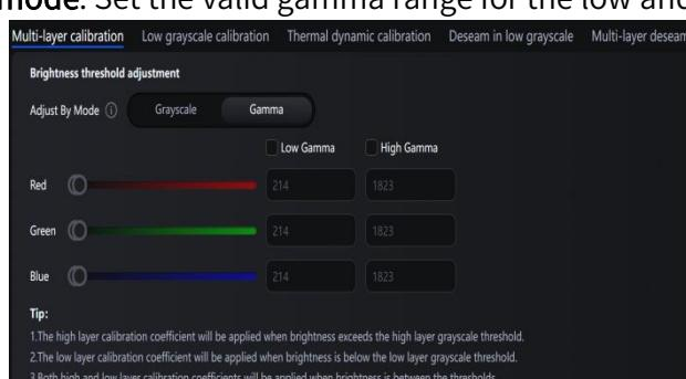
Fig 7.2.4.2 Multi-layer calibration - Gamma value mode
