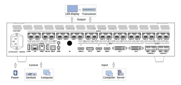
**Network port output**: When selecting the network port output, you can connect to the LED display through the network cable.
